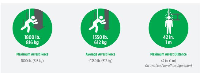
**Note:** Maximum Arrest Distance for foot-level tie-off does not have a stated limit and must be included in labeling and instructions.
